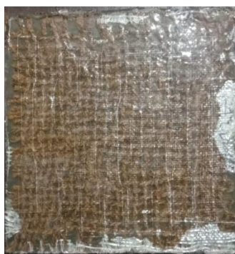
Gambar 5. Komposit Hybrid Hasil Curing
