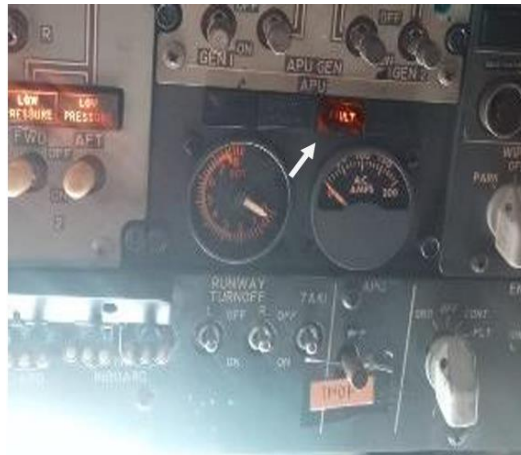
Gambar 5. Panel APU Fault
