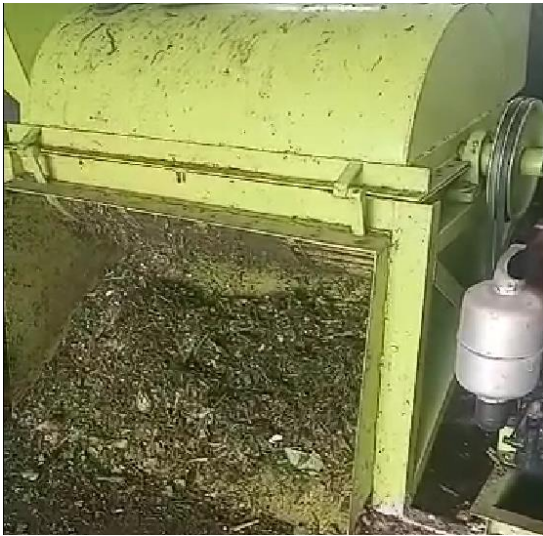
Figure 3. Small pieces of organic waste that comes out of an automatic waste sorting machine
